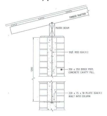
Figure 2 - The manner in which the pillar and tie down should have been constructed 3
