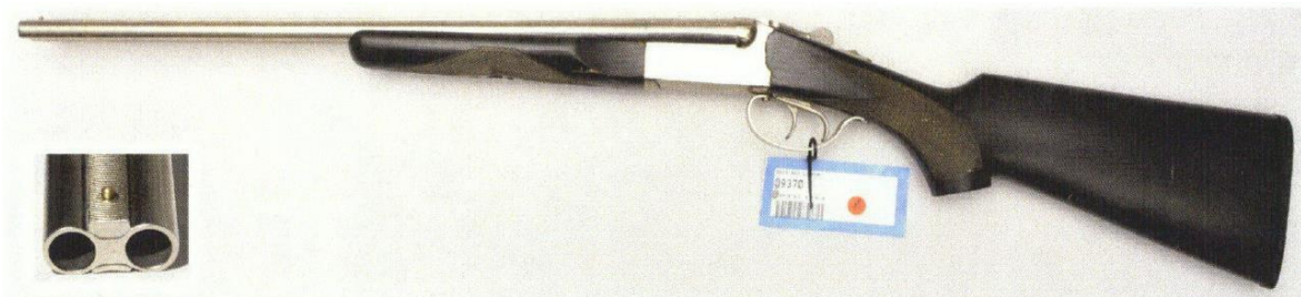
Figure 3. Showing profile of Firearms Reference Library shotgun, FRL ref 02313754, from left side (main picture) and barrel configuration from muzzle end (inset). Image JIP_6027 & 6033 - (cropped).
